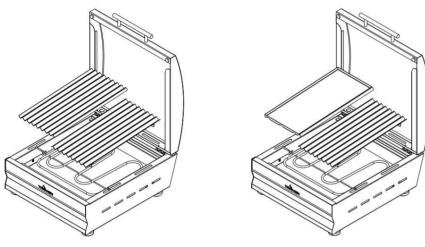
D) Remove the grease cup to wash it outside the equipment; use a soft sponge and hot, soapy water.Do not use steel shavings, or any sharp metal items, as they could be scratched.
