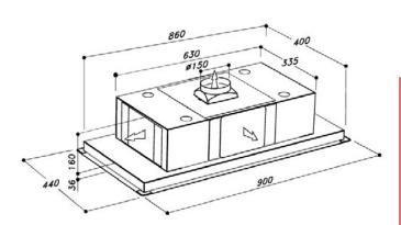
\*Outdoor offboard motors have a marine grade finish as standard for added resistance to coastal weather elements. \*Installation of this Rangehood must be centralised over the cooktop for optimum efficiency. This Rangehood can be installed over a 60-80cm cooktop at a 1600mm maximum height above the benchtop.
