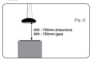
The cooker surface and the lowest part of the hood **must** be at a minimum distance, as shown above.
