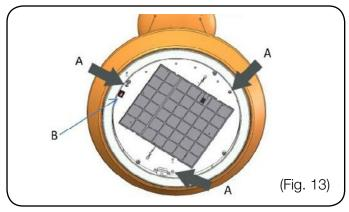
Using a Phillips screw head screwdriver, tighten or loosen the three screws in order to raise or lower the ceramic body on a specific side (fig. 14). After the adjustment insert the rubber tips and the grease filter again.
