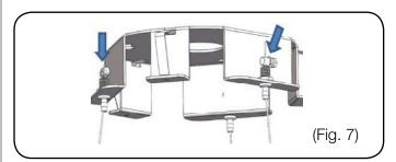
Put the hood near the ceiling and hook the plate to the screws previously installed (fig.8 A) Tighten the three screws fixing the plate to the ceiling, then block the hood definitively adding the security screw, see fig.9 B. Connect the appliance to the electric grid.
