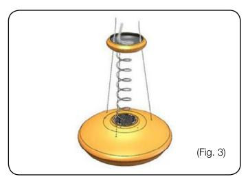
Take the metal plate from the packaging and then put the steel cables through the appropriate supports, as shown in Fig. 4.
