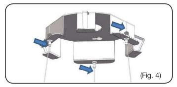
Adjust the height of the rangehood by scrolling the steel cables up and down inside the support. You need to unscrew and push the support in order to allow the scrolling of the cable, see Fig. 5.
