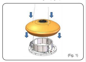
Put the power cable through the air outlet grill, see Figure 2. The ceramic part must perfectly cover the metal part named "D" in the exploded view.
