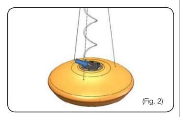
Extract from the packaging the ceramic cover for the ceiling plate (see the detail B on the exploded view), place the cover over the hood and put the steel cables through the three holes in the ceramic body, the power cable should be put through the central hole of the ceramic, see Fig.3.
