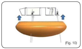
In case the ceramic cover of the body, is not perfectly flat or parallel to the body, it is possible to make an adjustment after installation. Remove the grease filter as described in Maintenance Section, remove the three plastic caps shown in Figure 13 A.
