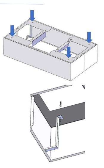
**3.** After installing the mount kit, proceed by making the holes to install the hood.
