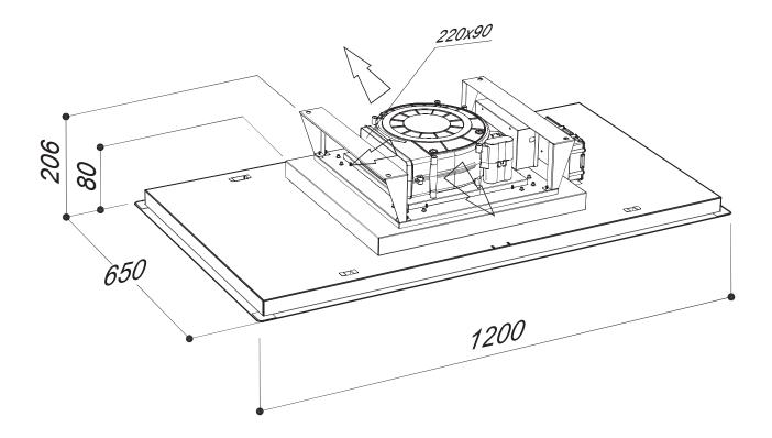
For the installation, create a false ceiling with a niche of 1165mm x 615mm with height between 200mm and 280mm
