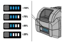
The indicator goes out after 3 seconds. If one of the LEDs flashes, the battery must be recharged. If none of the LEDs light up after the button is pressed, the battery is faulty and must be replaced.
