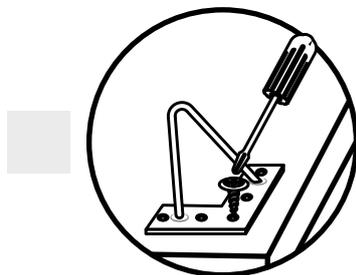
Your set includes four iron hairpin legs. To assemble these you will need a star type screwdriver or a power tool with a star type end. Holes for the legs has been pre-drilled and should be clearly visible underneath your record stand. Please align the base of hairpin legs along the pre drilled holes. Using a screwdriver or a power tool attach the legs with included screws.
