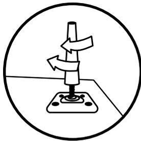
Your set includes four wooden legs. These need to be attached to the bottom part of your record stand. You can easily fit these by screwing them in with your hand. We have fitted the legs plates for you.
