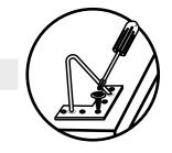
Your set includes four iron hairpin legs. To assemble these you will need a star type screwdriver or a power tool with a star type end. Holes for the legs has been pre-drilled and should be clearly visible underneath your record stand. Please align the base of hairpin legs along the pre drilled holes. Using a screwdriver or a power tool attach the legs with included screws.
