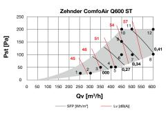
$L_w$  in dB(A) reference  $10^{-12}$ W, SFP [w/(m³/h)] calculated using data measured in accordance with EN 13141-7: 2010,  $^1L_w$  in dB(A); sound, supply air/extract air measured in accordance with ISO 3741 including end reflection in accordance with EN 13053:2006,  $^2$ Zehnder ComfoAir Q with G4/G4 filter and pre-heater
