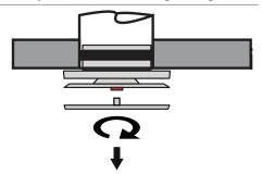
Turn the design cover a quarter counterclockwise and then remove it from the valve.
