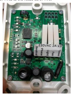
Do not over tighten the screw terminals!
