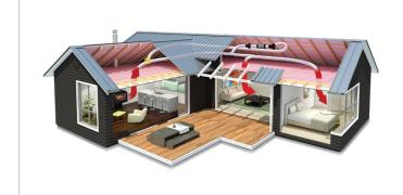
Integrated DVS® Premium Connect in Heat Transfer Mode
