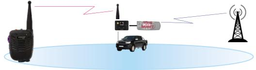
The gateway connects to your mobile radio in your vehicle (or office control station). It passes all voice traffic to and from the secure wireless microphone.
