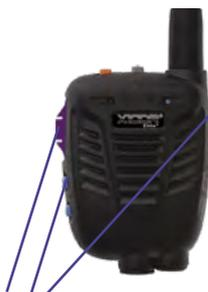
Turn Off handset and then press and hold PTT, Volume Up and On button until triple press sounds.
