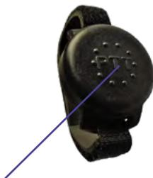
Triple press to turn Off PTT button. Wait 1-2 seconds and then press and hold PTT for 10 seconds.
