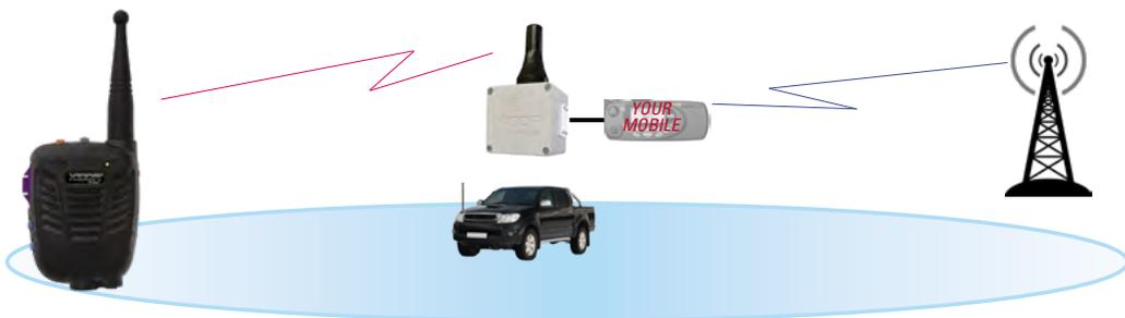
The gateway connects to your mobile radio in your vehicle (or office control station). It passes all voice traffic to and from the secure wireless microphone.
