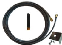
1 x XMCAK rack mount antenna kit (included) Includes 5.2m LMR200 type low loss coax terminated in RP-SMA connectors, right angle mounting bracket with screws.
