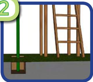
**Mark a point on the ground - 60cm away from your wooden construction. Dig a hole with a depth of 40cm for the fireman's pole to go into.**
