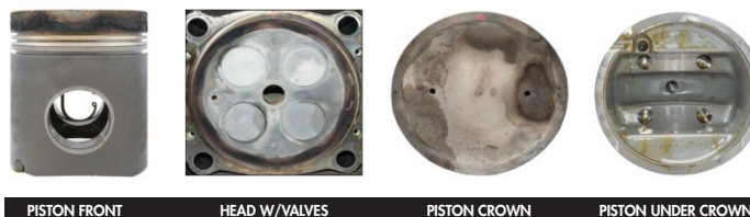
Maxima SNG 15W-40: Caterpillar G3612 Engine Test
