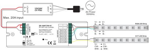
Note: please make sure the dip switches are at position for RGB+CCT mode as shown in above diagram.
