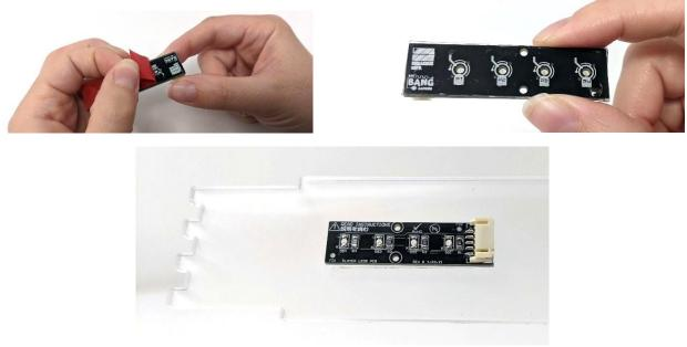
Apply power and see the results! Be sure to leave the Player LEDs PCB undisturbed for 24 hours to give the double-sided tape a chance to fully adhere and achieve maximum strength.
