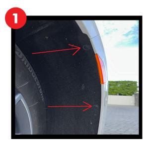
**STEP ONE:** REMOVE THE (2) STAR HEAD SCREWS ON THE FENDER APRON TO GAIN ACCESS TO THE INSIDE OF THE FENDER AREA.
