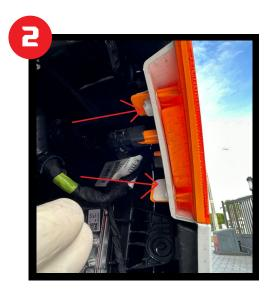
STEP TWO: PUSH THE TWO WHITE RETENTION TABS BACK THROUGH THE HOLDING CLIPS ON THE OEM FENDER LIGHT.
