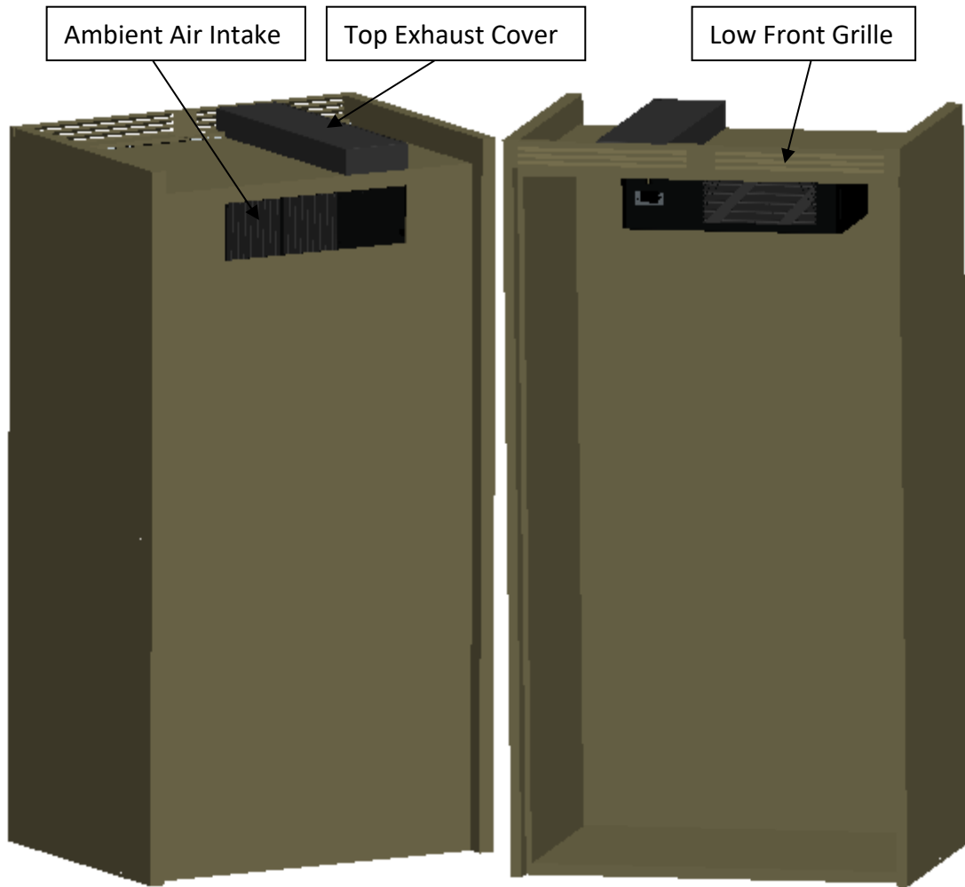
Fig. 2.9 Cooling Unit Installed (Low Front Grille)
