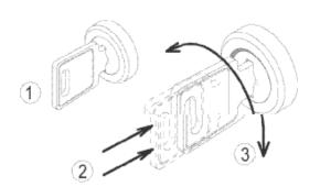
As a security measure, the lock on your wine cellar works on a double movement system. The key should be pushed inward and turned at the same time to operate.
