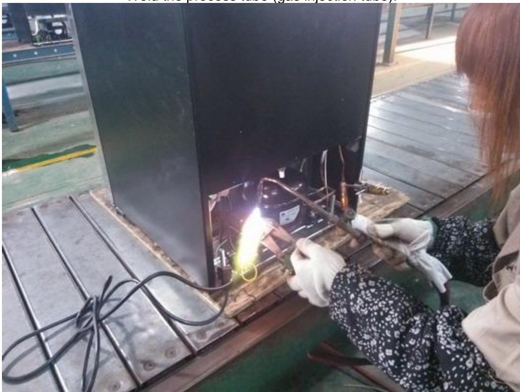
Nip the seal tube (on the dry filter body) and then weld its end.
