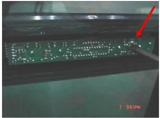
Using a screwdriver, remove the screws so that you may remove the control board from the door. Place these screws in a safe place for later use.
