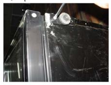
16. Upright the cabinet , install the upper door axis socket.(Attention: keep two sides of door and cabinet flat)
