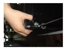
15. Install the feet kit into the bottom of the cabinet (the position the lower door axis accessory installed before)
