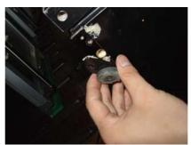
12. Take off the lower right door axis sleeve, and fit in the left door axis hole.
