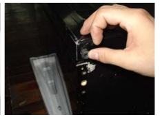
13. Install the lower door axis accessory to the left cabinet, and fix the door. (Attention: don't press the door gasket too tight)
