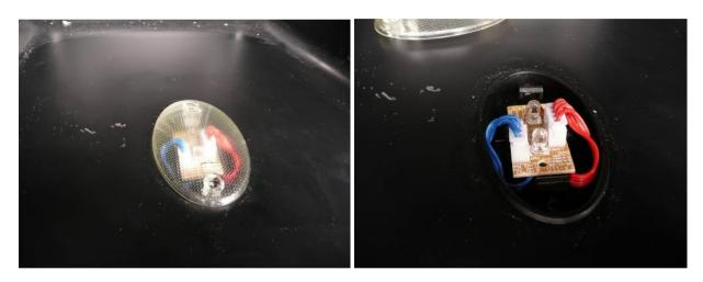
b. If the wires are in good condition, change the light power control board.
