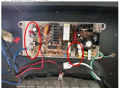
iii. Remove screws from the power control board.
