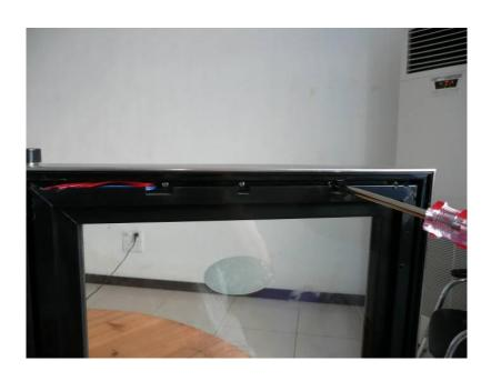
iii. Remove the temperature controller.
