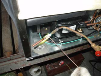
4-7-5、 Install the vacuumizing connector onto the process tube.
