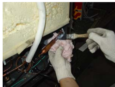
4-7-8、 Cover the welding point with towel that is soaked with soapsuds. If there is bubbles it means there is seam
