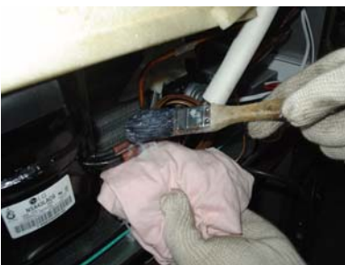
4-7-8、 Cover the welding point with towel that is soaked with soapsuds. If there is bubbles it means there is seam
