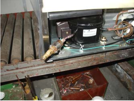
4-7-6、 Charge nitrogen. Connect the dried Nitrogen with the pressure is 1Mpa to the process tube
