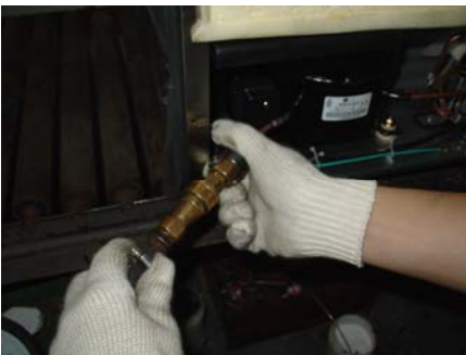
4-7-8、 Cover the welding point with towel that is soaked with soapsuds. If there is bubbles it means there is seam
