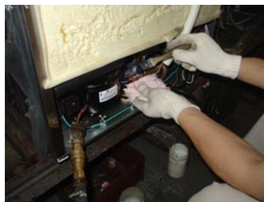
4-7-8、 Cover the welding point with towel that is soaked with soapsuds. If there is bubbles it means there is seam
