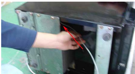
19、 Fix the new sensor in about 10cm, and do adjusting
