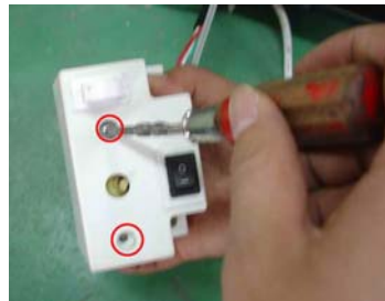
19、 Fix the new sensor in about 10cm, and do adjusting
