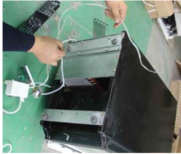
18、 Chang a new temperature controller, and fix it in the box
