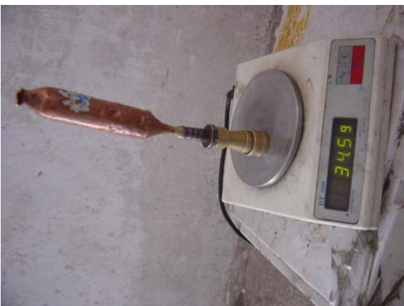
1-4-6-12、 Weigh the canned bottle after charging.
