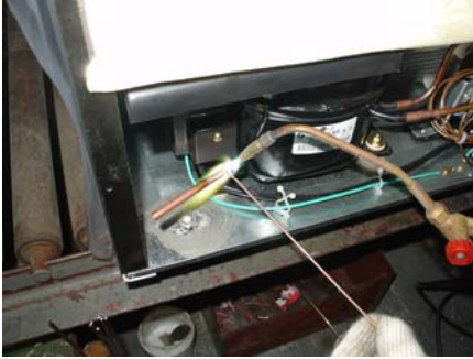
1-4-6-4、 Install the vacuumizing connector onto the process tube.
