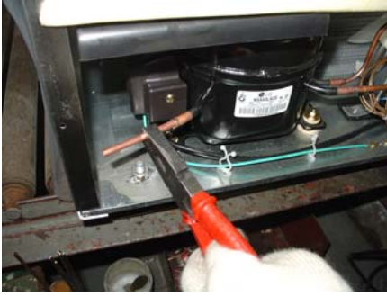
1-4-6-3、 Fix the process tube by welding.
