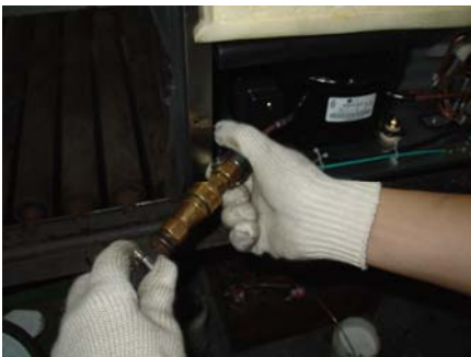
1-4-6-6、 Cover the welding point with towel that is soaked with soapsuds. If there is bubbles it means there is seam
