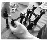
**3** Once all the metal supports have been inserted on this side, using a rubber or plastic mallet, tap in each metal part so they are inserted ALL the way into the polymer bottle rest. It is critical for safety reasons that all of these parts are inserted all the way in as far as they can go.
