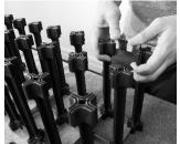
4 Turn the wine rack around and insert the metal supports into the second side of the polymer bottle rest by hand. Once all the metal components have been inserted, using the mallet, tap in each metal part so they are inserted all the way into the polymer bottle rest.
