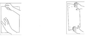
2. Drill 10 installation holes into the wall following the diagram on the sticker.
