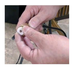
Connect the Glass Froster to the CO2 cylinder using the fitting supplied. Using a wrench, turn the nut clockwise until it is tight.
