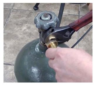
Next, open the gas flow using the knob located at the top of the CO2 cylinder. Please make sure that the CO2 cylinder sits vertically at all times. NOTE: Stand to the side of the cylinder when opening the cylinder valve. Open the cylinder valve slowly.
