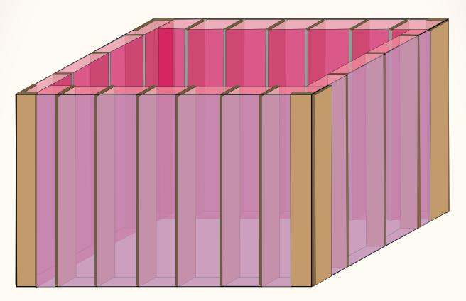
Use fiber glass, foam or blown-in insulation. A min of R-13 is required for walls, R-19 for the ceiling, but R-30 is recommended.
