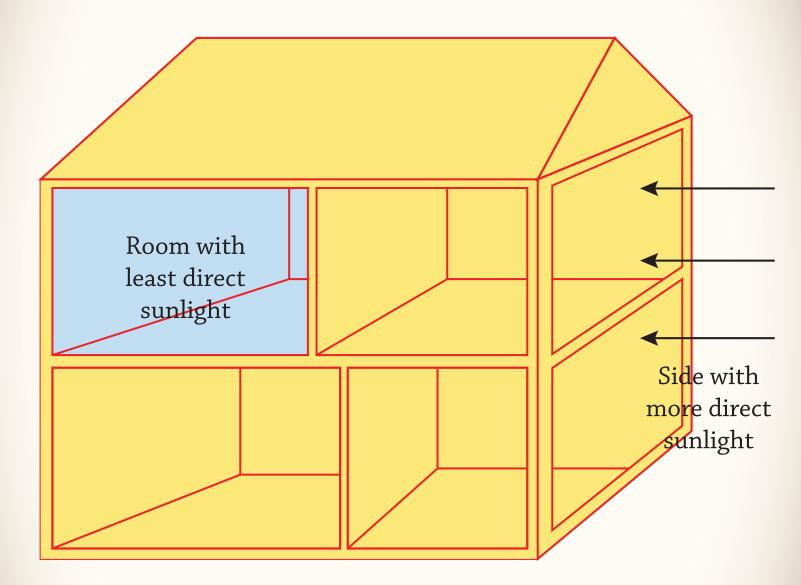
Choose an available room with the least amount of direct sunlight. The less heat it holds, the better your cooling unit and venting system will run.
