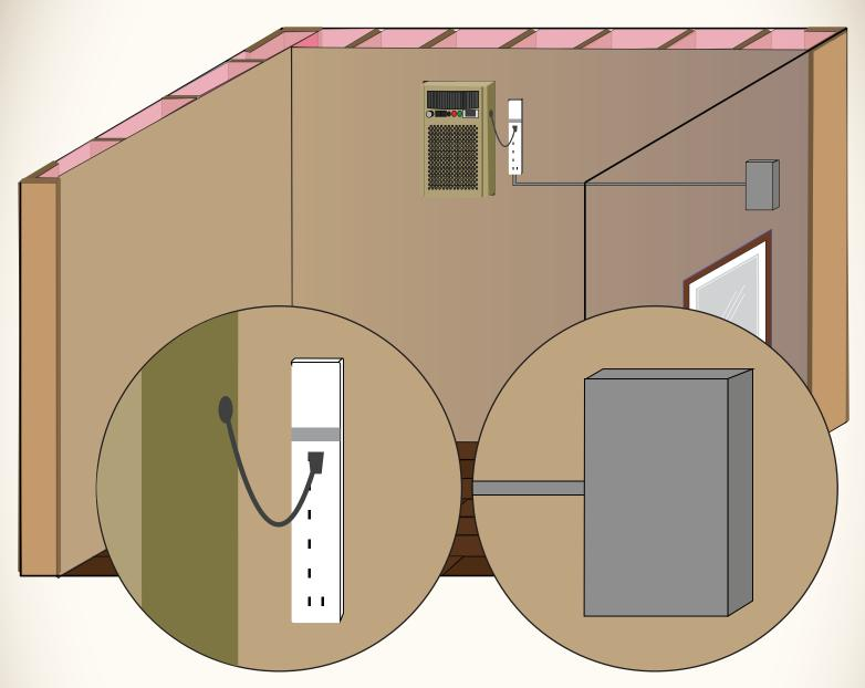
For safety, it is important to be familiar with the requirements of any electrical device you purchase. To hook up the system, plug in the front or back of the unit and be sure to use a surge protector. It will require a dedicated 110 volt, 20 AMP circuit.
