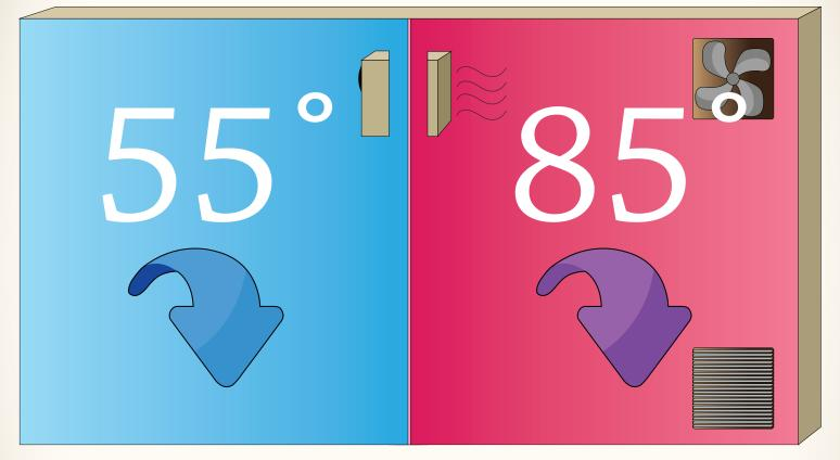
The MAXIMUM temperature difference between your wine cellar and exhaust room should only be 30°. A good cooling unit will regulate temperature fluctuations.
