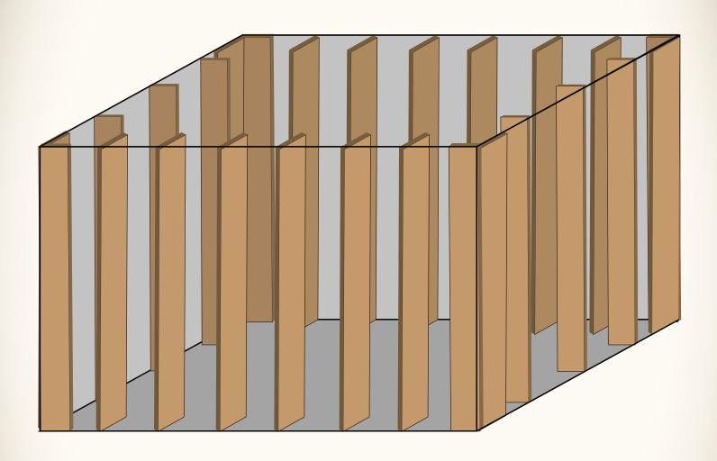
Use 2x4 or 2x6 construction. The more you insulate the cellar, the cooler it will be.
