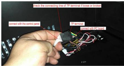
4. Check if the control panel is faulty, replace by another new control panel. If the display is working normally, that means the old ones is faulty.
