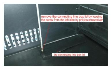
3. Check the connecting line of 7P terminal if loose or broken
