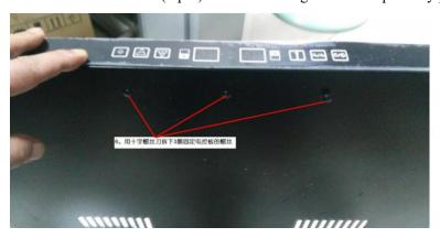
7. Loosen the control panel, remove the screws (5 pcs) by phillips screwdriver, keep the
