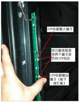
4. Disassemble the screws (3 PCS) to remove the light panel, and use these 3 screws to fix the light panel after replacing with the new light panel.
