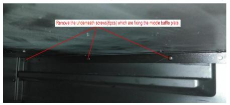
3. Pull out the middle baffle plate.
