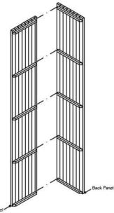
Step 1: (Attaching side panel to back panel)
