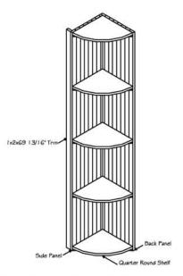
Step 3-Optional: (Attaching the  $1x2x69!\frac{3}{4}6"$  trim) Since the QR-G is not as deep as the other Apex Modular Racks, Apex has provided a  $1\times2\times69^{1}\%$  long trim board as an optional piece when mounting the QR-6 to another modular rack. The trim board is used to fill in the gap
