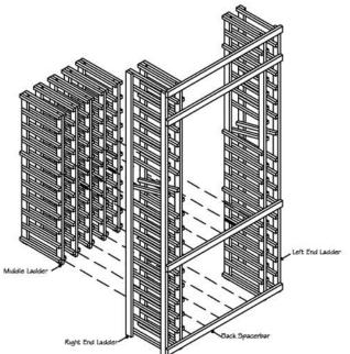
Step 3: (Attaching the 39" tall middle ladders) Insert the five 39" tall middle ladders into the slots of the spacerbar as shown. Nail each middle ladder onto the spacerbars as shown with the nails provided.
