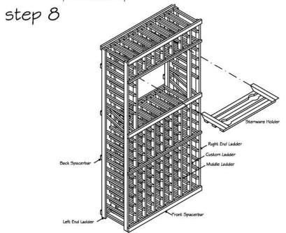
into place. Screw the stemware holder in each of the four corner through the custom ladders.
