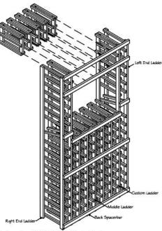
Step 5: (Attaching the 8 3/16" tall middle ladders) Insert the five 8 3/16" tall middle ladders into the slots of the spacerbar as shown. Nail each middle ladder onto the spacerbars as shown with the nails provided.
