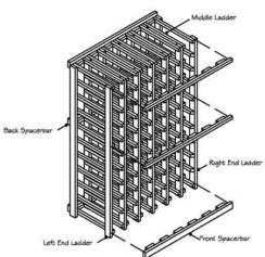
Step 3: (Attaching Ix2 \* Ix1 front spacerbars)
