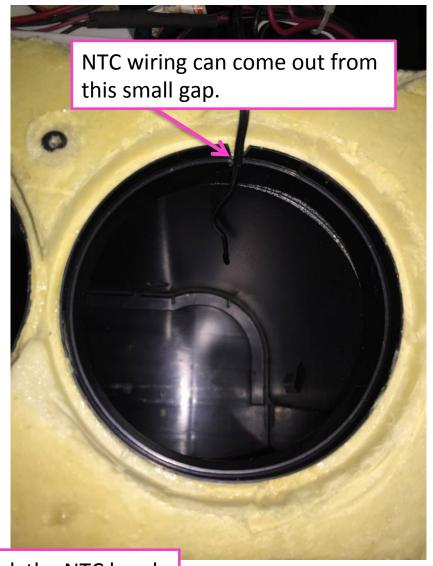
Use the Aluminum foil paper to stick the NTC head onto the aluminum back wall.
