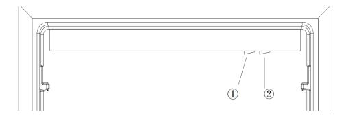
Light switch positions are located inside the unit (shown above) for you to turn the backlight on/off.
