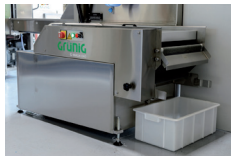
Closed circuit tank with inclined filter
