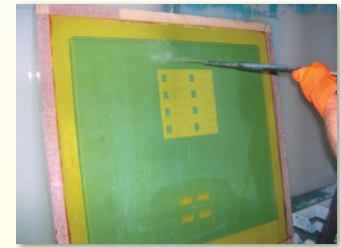
3. High pressure rinse - starting at bottom.
