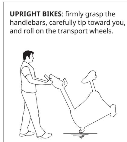
**UPRIGHT BIKES:** firmly grasp the handlebars, carefully tip toward you, and roll on the transport wheels.
