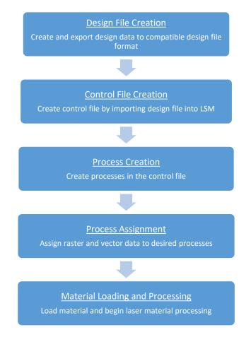
ULTRA R5000 and R9000 Laser Material Processing Workflow
