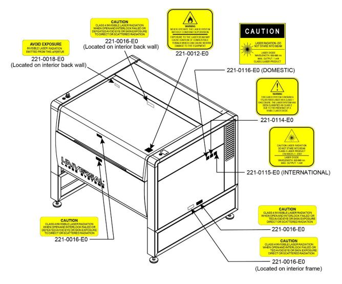
ULTRA R5000 and R9000 Platforms Safety Labels (Isometric Side View)
