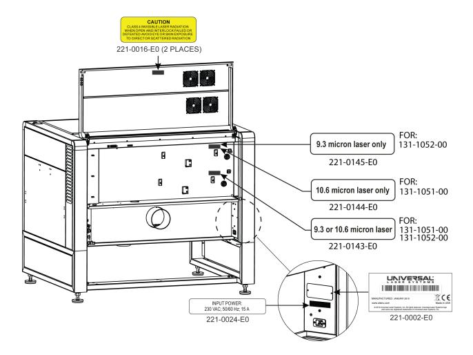
ULTRA R5000 and R9000 Platforms Safety Labels (Rear View with laser cover open)
