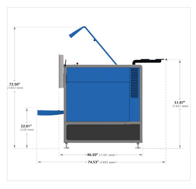
ULTRA R5000 and R9000 Platform with optional Touch Screen Control Panel (Side View) All dimensions are indicated in inches and millimeters.
