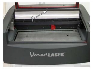
**4.** Rotate the cover (1) up and over the top of the X-axis Arm. The cover is held down by magnets and will "stick" slightly when you first begin to pull it upward.
