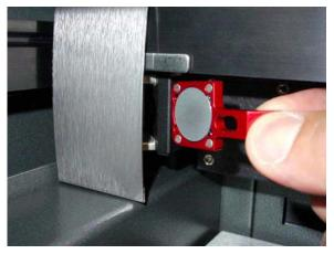
7. Install the new Mirror 2 by sliding it into the mounting slot until it stops. Installing NOTE: the mirror backwards will cause the handle to protrude in such a way that the X-axis Arm cover will not close properly and will destroy the mirror once the laser beam penetrates the backside of the mirror, so be sure that you reinstall the mirror correctly.
