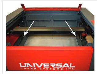
**2.** Open the top door and bring the X-Axis Arm forward.
