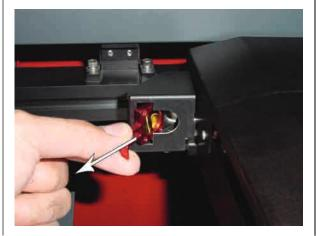
3. Locate the #2 Mirror holder (red). Grasp its protruding handle with your thumb and forefinger and slide it out. It is held in place by magnets so you may feel a slight resistance when you begin to slide it out.
