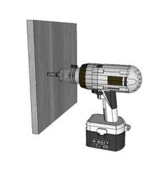
Faster Installation Method: Purchase an anchor bolt driver: fit the anchor bolt driver into an electric drill, screw anchor bolt into driver and then drill into your pilot hole. Be careful not to screw too deep. Leave sufficient bolt length sticking out of the wall for mounting the peg.
