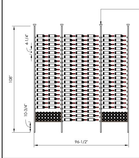
Telescopic bracket allows height to be extended up to 112"
