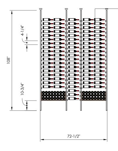
Telescopic bracket allows height to be extended up to 112"
