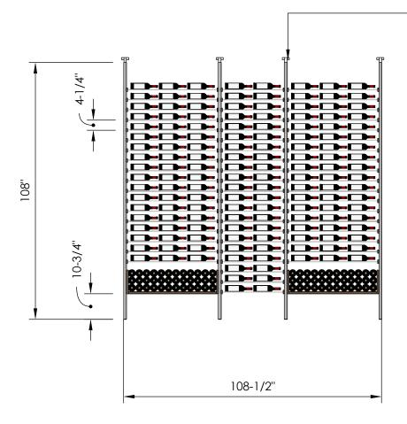
Telescopic bracket allows height to be extended up to 112"
