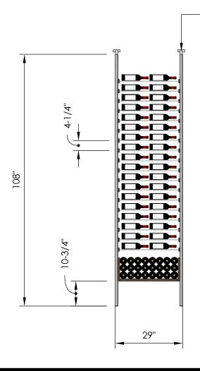
• Telescopic bracket allows height to be extended up to 112" (Post can be cut down by up to 4 inches for a racking height as low as 104")
