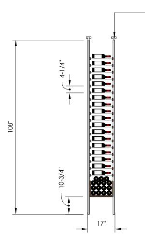
Telescopic bracket allows height to be extended up to 112"
