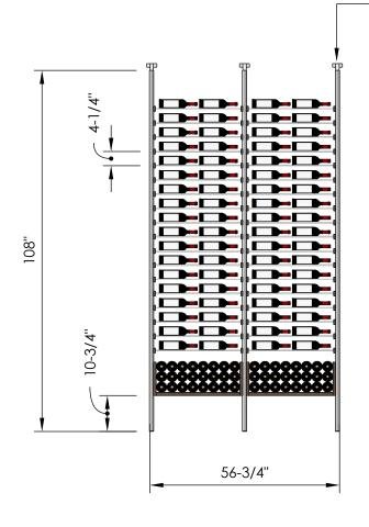
Telescopic bracket allows height to be extended up to 112"
