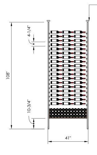
• Telescopic bracket allows height to be extended up to 112" (Post can be cut down by up to 4 inches for a racking height as low as 104")
