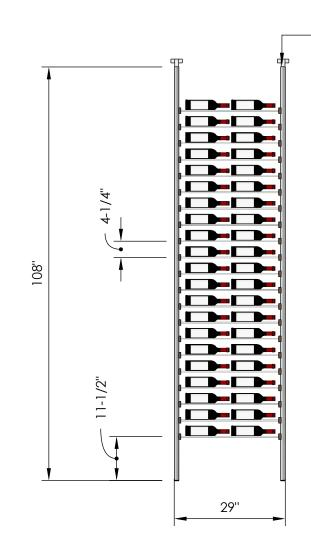
Telescopic bracket allows height to be extended up to 112" (Post can be cut down by up to 4 inches for a racking height as low as 104")
