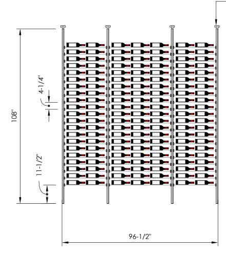
Telescopic bracket allows height to be extended up to 112" (Post can be cut down by up to 4 inches for a racking height as low as 104")
