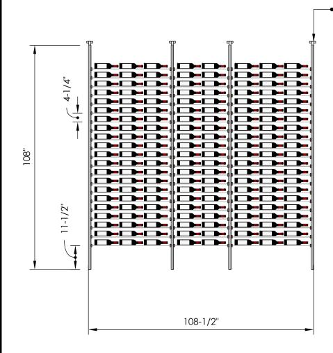
• Telescopic bracket allows height to be extended up to 112" (Post can be cut down by up to 4 inches for a racking height as low as 104")
