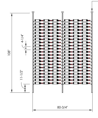
Telescopic bracket allows height to be extended up to 112" (Post can be cut down by up to 4 inches for a racking height as low as 104")
