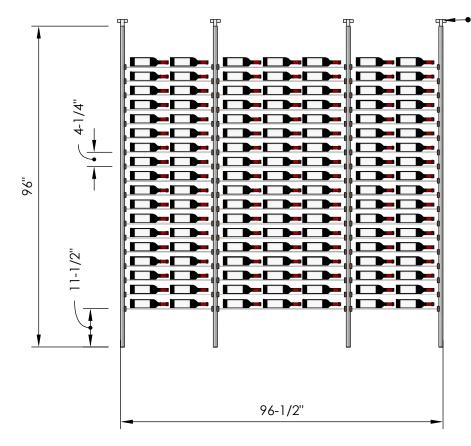
Telescopic bracket allows height to be extended up to 100" (Post can be cut down by up to 4 inches for a racking height as low as 92")
