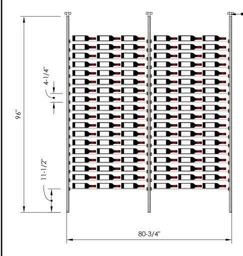
Telescopic bracket allows height to be extended up to 100" (Post can be cut down by up to 4 inches for a racking height as low as 92")
