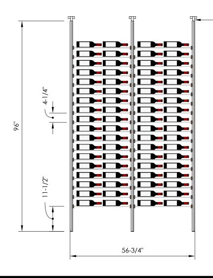
Telescopic bracket allows height to be extended up to 100" (Post can be cut down by up to 4 inches for a racking height as low as 92")
