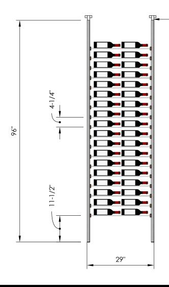
Telescopic bracket allows height to be extended up to 100" (Post can be cut down by up to 4 inches for a racking height as low as 92")
