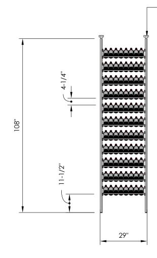
Telescopic bracket allows height to be extended up to 112" (Post can be cut down by up to 4 inches for a racking height as low as 104")
