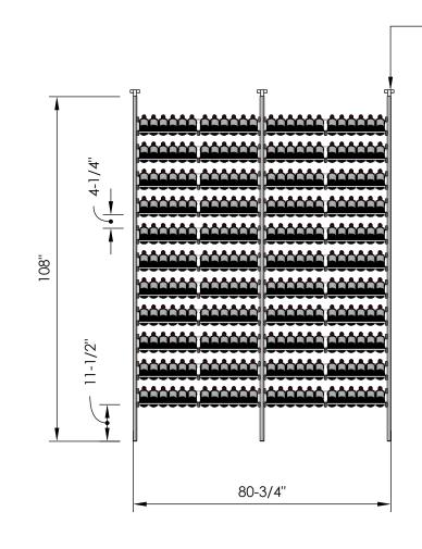
Telescopic bracket allows height to be extended up to 112" (Post can be cut down by up to 4 inches for a racking height as low as 104")
