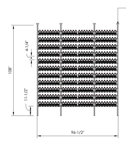
Telescopic bracket allows height to be extended up to 112" (Post can be cut down by up to 4 inches for a racking height as low as 104")
