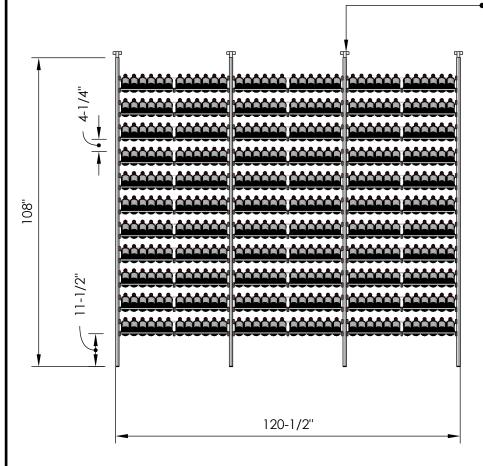
Telescopic bracket allows height to be extended up to 112" (Post can be cut down by up to 4 inches for a racking height as low as 104")
