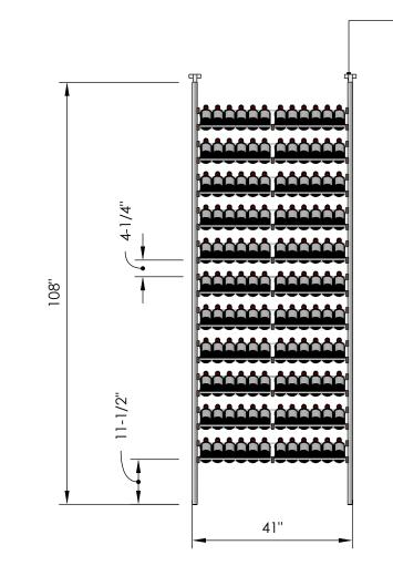
Telescopic bracket allows height to be extended up to 112" (Post can be cut down by up to 4 inches for a racking height as low as 104")
