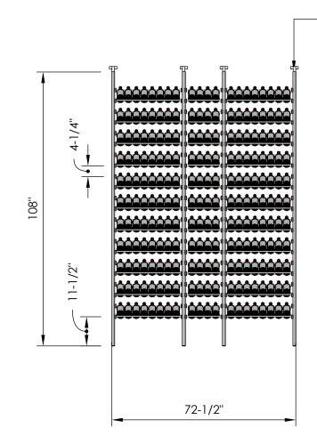
Telescopic bracket allows height to be extended up to 112" (Post can be cut down by up to 4 inches for a racking height as low as 104")
