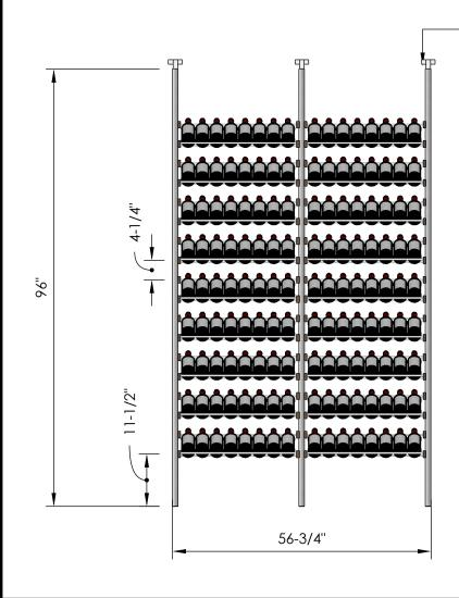
Telescopic bracket allows height to be extended up to 100"
