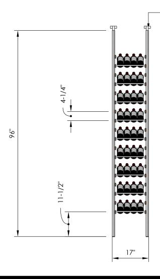
Telescopic bracket allows height to be extended up to 100"
