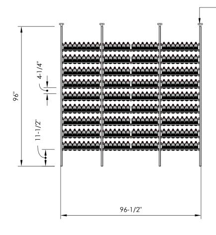
Telescopic bracket allows height to be extended up to 100"
